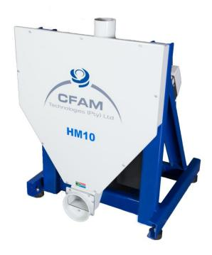
The CFAM HM 10 fine granulation hammer mill features a teardrop screen design with a replaceable grinding plate. The teardrop design stops the product from rotating with the rotor thus improving the grinding efficiency while the replaceable grinding plate reduce the impact stress on the screen.
