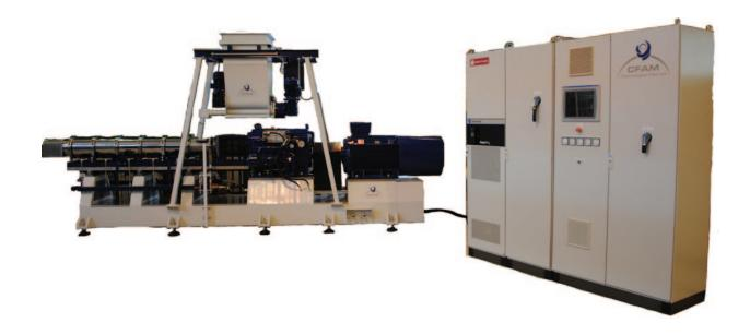
Extruder type: Co-rotating, fully intermeshing
